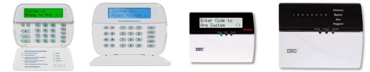
ARMING IN STAY MODE: With the green ready light on (all zones closed) press and hold STAY until it beeps. Motion Detectors will automatically be bypassed.
